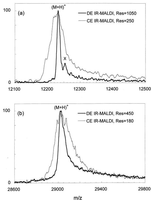
**Figure 2.** Comparison of CE and DE IR-MALDI mass spectra showing the singly protonated  $(M+H)^+$  regions of (a) bovine cytochrome *c* and (b) bovine carbonic anhydrase II. Matrix: sinapic acid. The peak labeled X is located  $21.0 \pm 1.0$  Da above the  $(M+H)^+$  ion peak. “Res” designates the full width at half maximum resolution.
