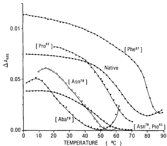
Figure 8. Plots of the change in absorbance at 695 nm with increasing temperature for cytochrome c and its analogues. Sample solutions were made up in 10 mM sodium cacodylate, 10 mM sodium chloride, pH 7. Absorbance measurements were made at 2° intervals over all or part of the range 0-90°. These data were used to construct the Arrhenius plots shown in Figure 5 from which the T<sub>1/2</sub> and thermodynamic parameters shown in Table 3 were calculated.
