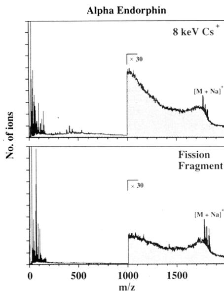
**Figure 3.**  $\alpha$ -Endorphin (1746 u) positive ion spectra: upper, 8-keV  $\text{Cs}^+$  ion bombardment; lower,  $^{252}\text{Cf}$  fission fragment bombardment.
