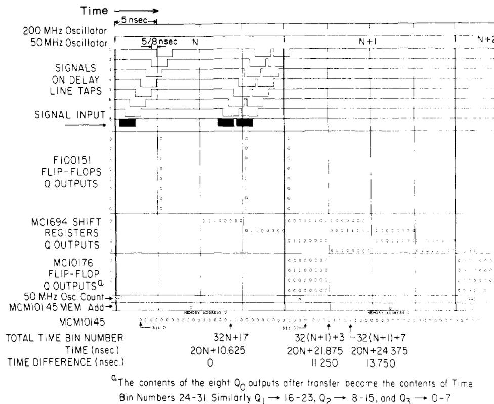
Figure 2. Time sequence and bit pattern flow.
