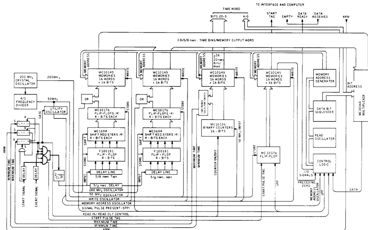
Figure 3. Summary diagram—components, interconnections, and data flow.
