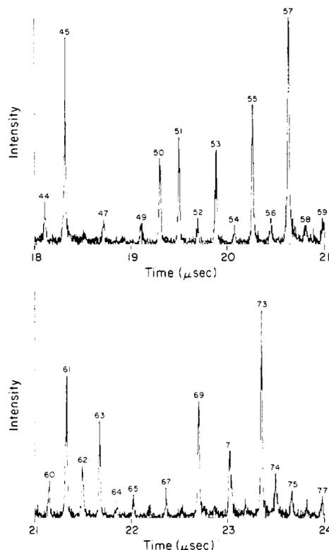
Figure 5. Portion of positive ion spectrum of sucrose.
