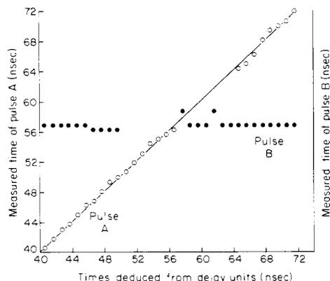
Figure 4. Test of high-resolution portion of timer—measured vs. known pulse times.
