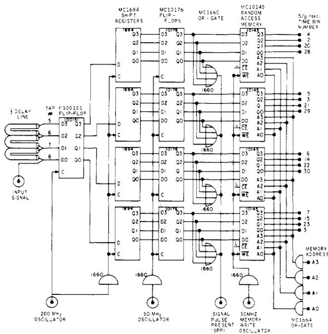
Figure 1. Half of the high-resolution portion of the time recorder.
