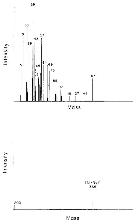
Figure 6. Complete positive ion spectrum of sucrose in histogram form.
