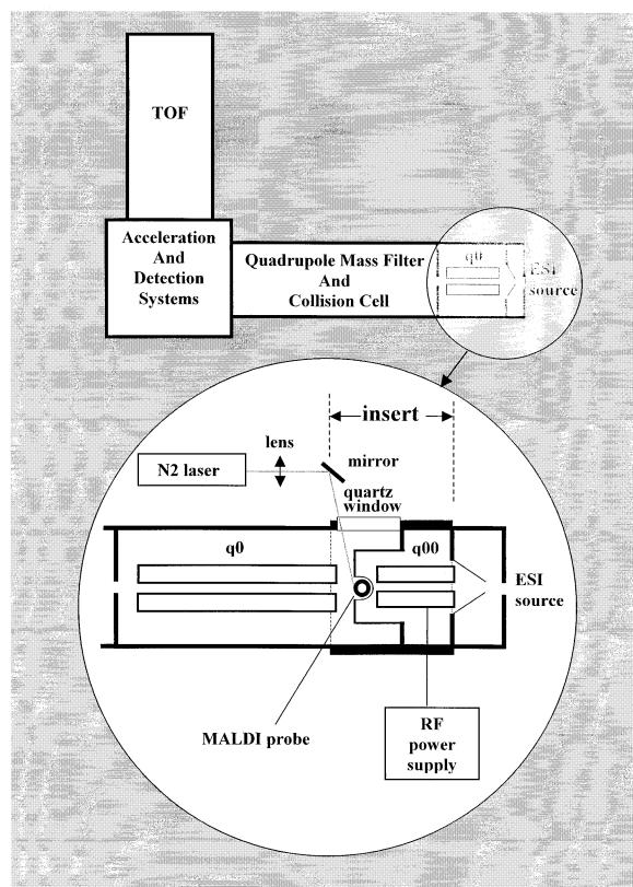
**Figure 1.** Schematic diagram of the prototype QqTOF mass spectrometer (Centaur, Sciex, Canada). The new interface is shown.
