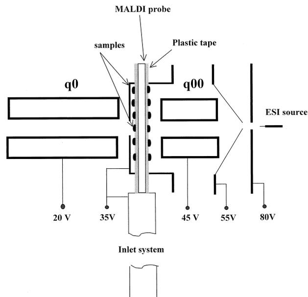
**Figure 2.** Distribution of voltages on the main elements of the ion optics in the new interface.
