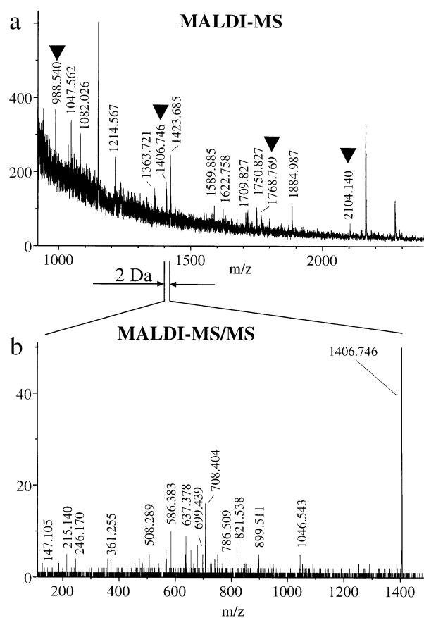
**Figure 6.** (a) MALDI-MS tryptic map obtained from  $\leq 5$  fmol of a  $\sim 70$  kDa protein from *S. pneumoniae*. (b) MALDI-MS/MS spectrum of the singly charged  $m/z$  1406.746 ion from the tryptic map.
