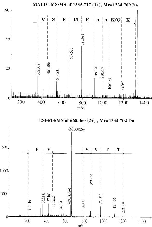
**Figure 10.** (a) MALDI-MS/MS of the singly charged tryptic fragment at  $m/z$  1335.717. The observed ladder of b-type fragments defines a 9-residue stretch of the amino acid sequence, i.e., ... VSE[I/L]EAA[Q/K]K. (b) ESI-MS/MS of the doubly charged ion at  $m/z$  668.360, arising from the same tryptic fragment as in (a). A short stretch of sequence can be deduced from the ladder of y-type fragments, i.e., ... TFVS, which is complementary to the sequence deduced from the MALDI-MS/MS spectrum.
