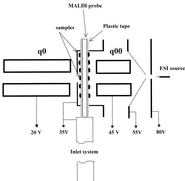
**Figure 2.** Distribution of voltages on the main elements of the ion optics in the new interface.
