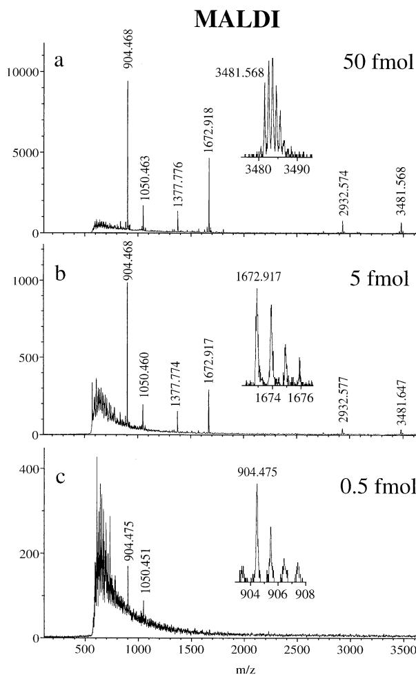
**Figure 4.** MALDI spectra of the six peptide calibration mixture discussed in the legend to Figure 3. The amount of sample applied to the probe is indicated. Spectra acquisition time = 1 min.
