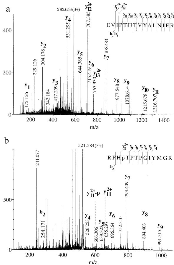
**Figure 11.** (a) ESI-MS/MS spectrum of a triply charged tryptic fragment ( $m/z$  585.653) from p42. Fully, 13 out of 15 residues in the peptide were identified from the  $y$ -fragment ladder. (b) ESI-MS/MS spectrum of the triply charged fragment at  $m/z$  521.584. The mass difference of 97.982 between the two doubly charged fragments at  $m/z$  655.297 and 606.306 indicates that the peptide is phosphorylated. PepFrag identified the origin of this phosphorylated peptide as htra2-beta3 [34].
