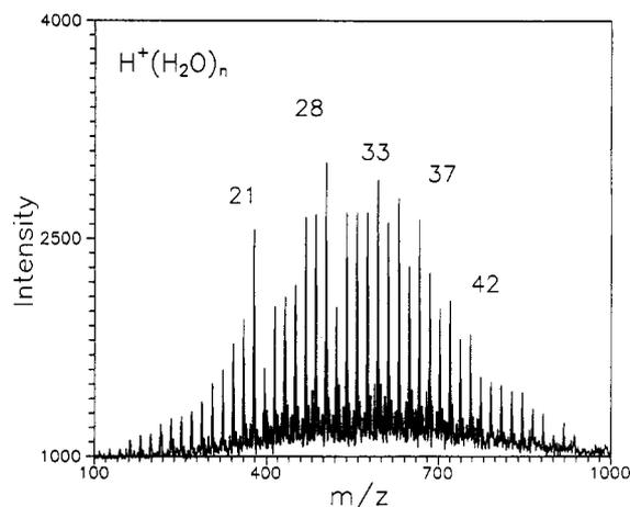
**Figure 2.** Electro spray ionization mass spectrum of water containing 1.0% acetic acid. The transport capillary tube was heated to 80 °C. The number ( $n$ ) on an ion peak denotes the number of water molecules attached to H<sup>+</sup>. Flow rate = 0.2  $\mu\text{L}/\text{min}$ . The spectrum is an average of 26 scans each acquired in 28 s.
