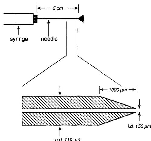
Figure 1. Shape and dimensions of a specially modified spray needle used for the electrospray of water, acidified water, and aqueous protein solutions.
