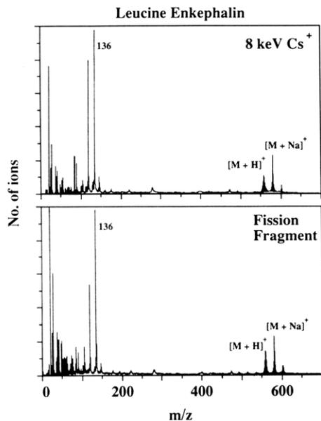
**Figure 1.** Leucine-enkephalin (556 u) positive ion mass spectra: upper, 8-keV  $\text{Cs}^+$  ion bombardment; lower,  $^{252}\text{Cf}$  fission fragment bombardment.
