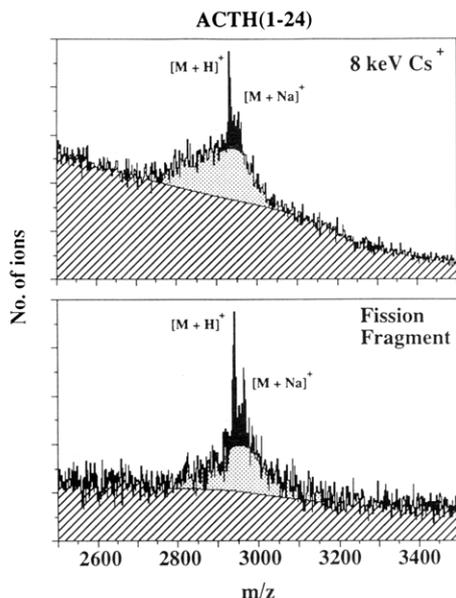
**Figure 6.** Quasi-molecular ion region of the positive ion spectrum for ACTH (1–24) (2933 u): upper, 8-keV  $\text{Cs}^+$  ion bombardment; lower,  $^{252}\text{Cf}$  fission fragment bombardment. The portion of the peak shaded black is interpreted as the quasi-molecular ion yield in Figure 5.
