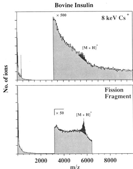
**Figure 4.** Bovine insulin (5733 u) positive ion spectra: upper, 8-keV  $\text{Cs}^+$  ion bombardment; lower,  $^{252}\text{Cf}$  fission fragment bombardment. Fission fragment data were taken up to  $m/z$  6500.
