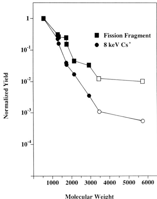
**Figure 7.** Relative yields as a function of molecular weight using the broad components of the quasi-molecular ion peaks for incident fission fragments (squares) and incident 8-keV  $\text{Cs}^+$  ions (circles). (The broad component for ACTH (1–24) is shaded gray in Figure 6.) Postacceleration was used for the data points depicted with open symbols; no postacceleration was used for the filled symbols.
