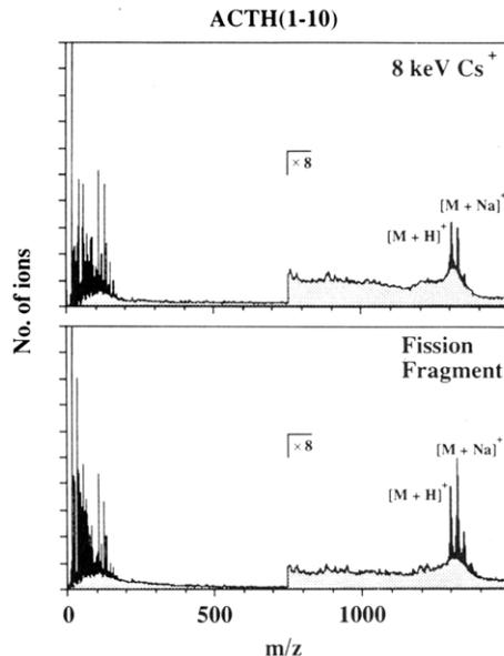
**Figure 2.** ACTH (1–10) (1299 u) positive ion spectra: upper, 8-keV  $\text{Cs}^+$  ion bombardment; lower,  $^{252}\text{Cf}$  fission fragment bombardment.
