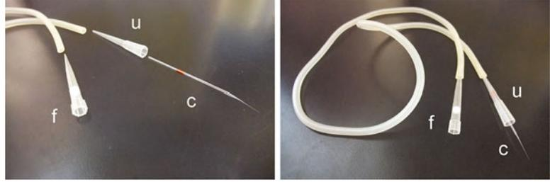
**Fig. 1** The pheromone delivery system. The filtered tip (f) connects the *upper end* of the tubing to the mouth and prevents saliva from going into the tubing. The unfiltered tip (u) connects the *lower end* of the tubing to the drawn-out glass microcapillary that contains pheromones diluted in M13 buffer (c)
